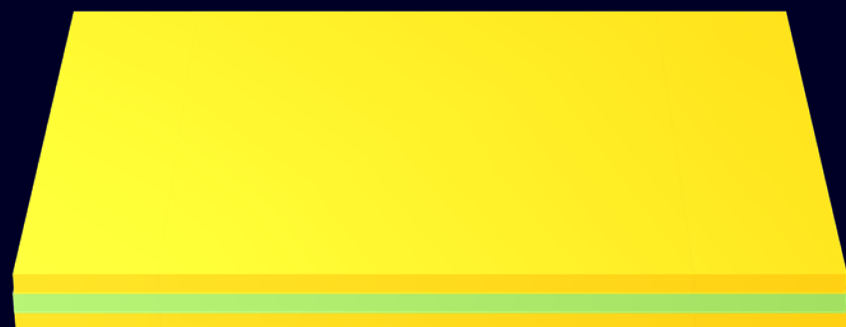
Au on both sides of Si 3 N 4 membrane
