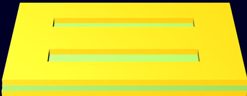
Alternating Gold slits removed by FIB
